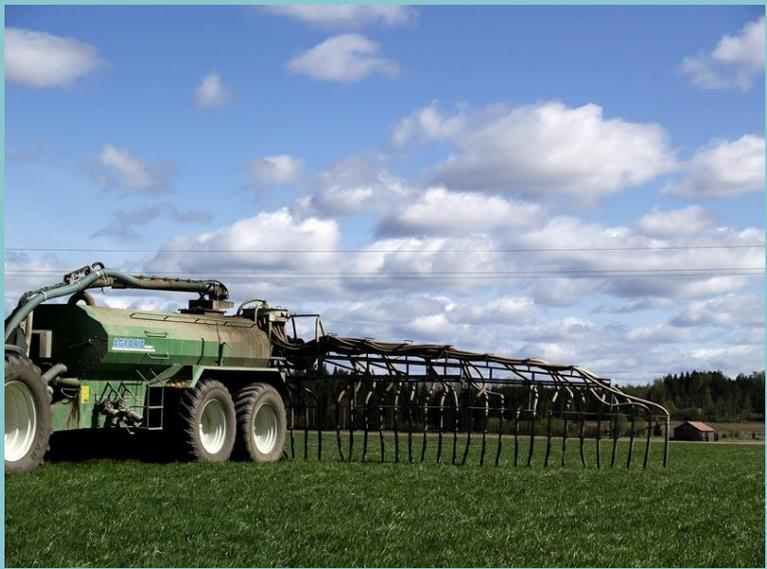
**Injection of liquid manure in soil (quite rare) into 6-10 cm depth reduce P losses**
